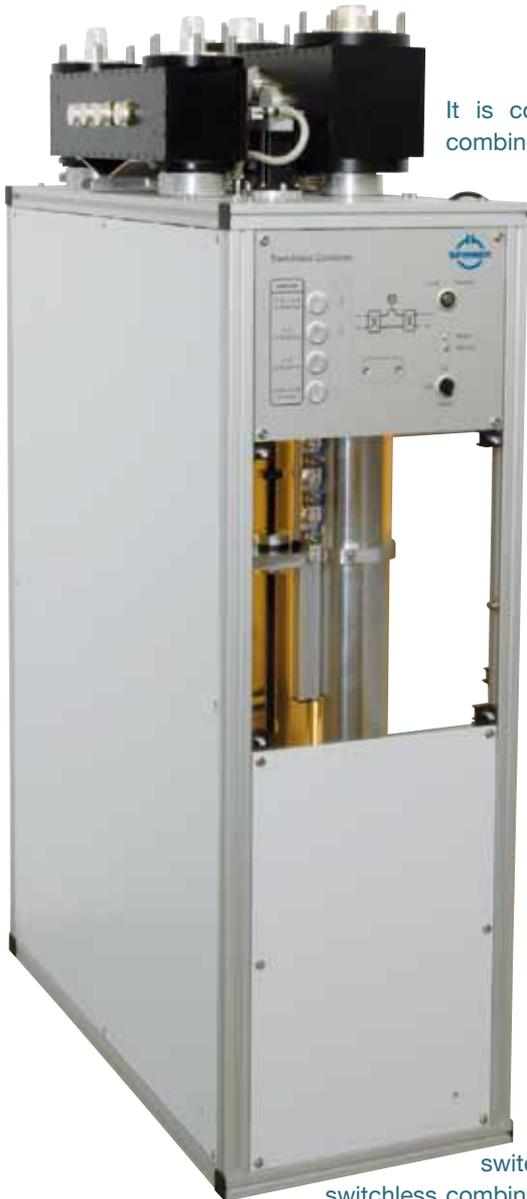
It is common practice to combine the power of two transmitters via 3 dB couplers to get double output power for normal operation.
