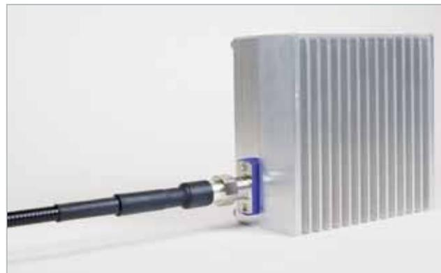
Low PIM jumper and load for measurement
