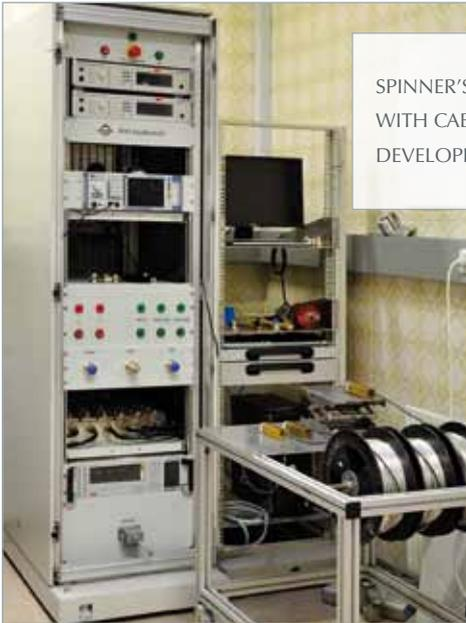
SPINNER'S FIRST PIM TEST BENCH WITH CABLE LOADS, CONTINUOUSLY DEVELOPED SINCE MORE THAN 20 YEARS
