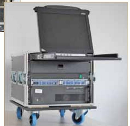
Thanks to the compact configuration, for the first time, a low cost DAB/DRM+ transmitter is therefore available for local operators and citizens' radio, for demonstrations and field tests. The functionality of the transmitter was demonstrated in the scope of the "entry into the digital distribution via
