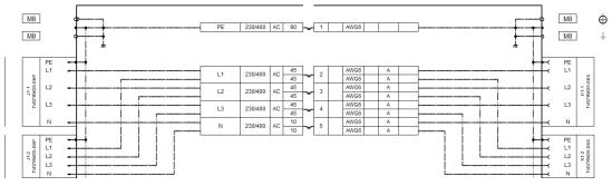
PE or shield paths of different groups may be interconnected through connections to the common housing of the slip ring.
