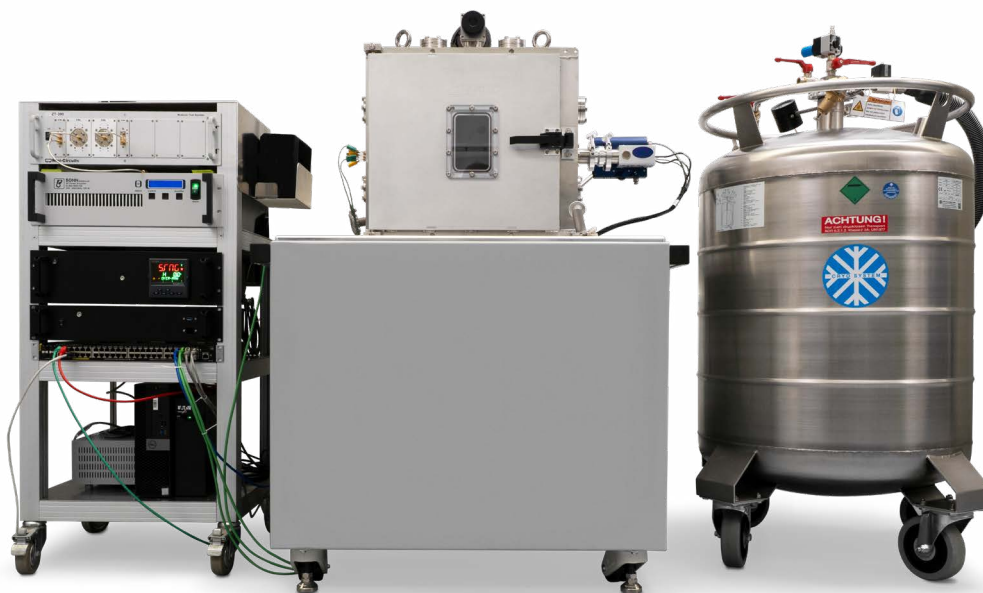
SPINNER uses its own vacuum chamber for Thermal Vacuum Tests (TVAC) to simulate the harsh conditions of space, focusing primarily on vacuum and extreme temperatures
