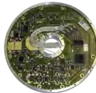
Ethernet Subassembly, Rotor Side, Small Version
