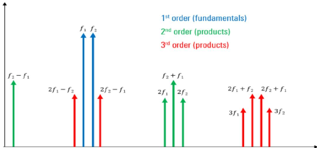
The "order" of intermodulation products refers to the sum of the coefficients. For example,  $2f_1$ , the second harmonic of  $f_1$ , is "second" order. Also the sum of the two fundamentals,  $f_1 + f_2$  is second order (1 + 1). The third harmonic of  $f_1$ ,  $3f_1$  is third order. And  $2f_2 - f_1$  or  $2f_2 + f_1$  are also third order products. These third order intermodulation products are particularly important when it comes to understanding passive intermodulation.
