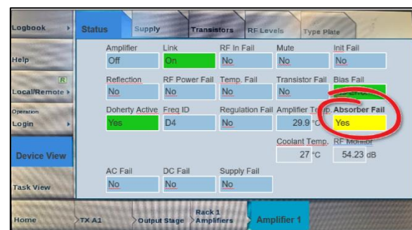
Transmitter GUI indicating float switch is working correctly if turned up side down
